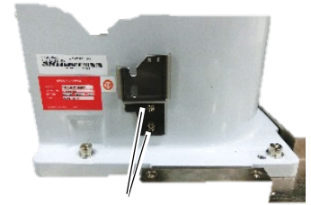
Hexagon socket head cap bolt 2-M4×10
