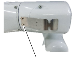
Hexagon socket head cap bolt 2-M4×10
