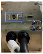
3. Connect the brake release unit to the connector of the connection cable.
