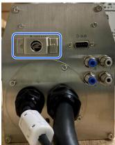
4. Connect the brake release unit to the connector of the connection cable.
