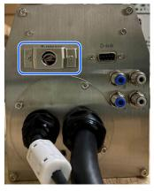
4. Connect the brake release unit to the connector of the connection cable.
