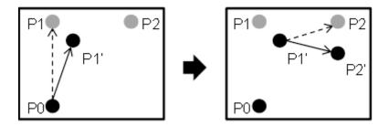
In the first Move, a trajectory from the initial position P0 to the target position P1 is planned (dashed line), and then the robot start motion.
