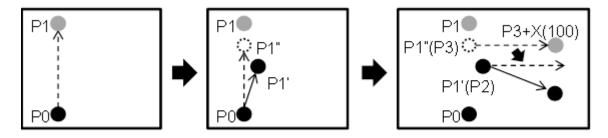
The stop position P1" on the planned trajectory at the time of motion stop by Till will be P3. The amount of relative displacement as position control can be specified based on P3.
