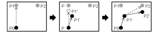
In the first Move, a trajectory from the initial position P0 to the target position P1 is planned (dashed line), and then the robot start motion.
