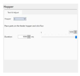
5. Adjust the volume of the hopper controller to make the parts move smoothly and at a constant speed. Adjust the duration so that the optimal number of parts are fed per click of the [Run] button.
