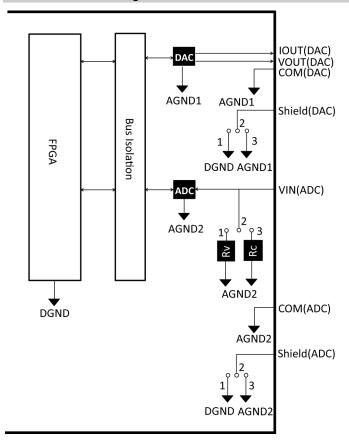
Rv: Voltage Input Terminating Resistance (100k $\Omega$ ),
