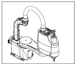
(2) Secure the base to the base table with four bolts. Be sure to use washers.
