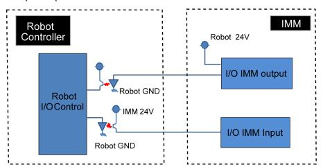
■ Input/output circuits do not have a built-in protection circuit to prevent short circuits or reverse connections.
