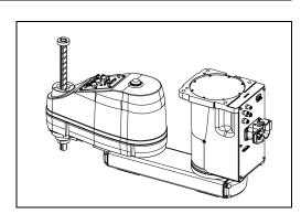
(2) Secure the base to the ceiling with four NOTE bolts. Make sure to use the washer.
