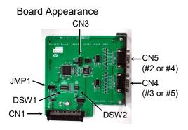
Switch and Jumper Configuration Set DSW1, DSW2 and JMP1. CN3 is all open.
