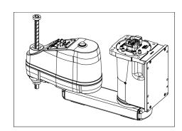
(2) Secure the base to the wall with four bolts. Make sure to use the washer.
