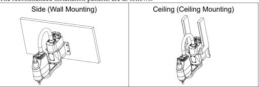
The recommended installation patterns for wall mounting are as follows:
