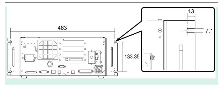
• To ensure proper ventilation around the supply and exhaust ports, install the Controller at a position that is the following distance away from other equipment and walls.
