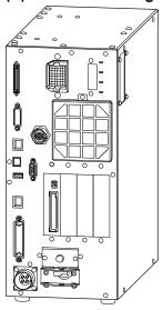
\* The rubber feet on the bottom need to be replaced. Attach the rubber feet with the flat side facing the Controller. Remove the screws that contact the rubber feet.
