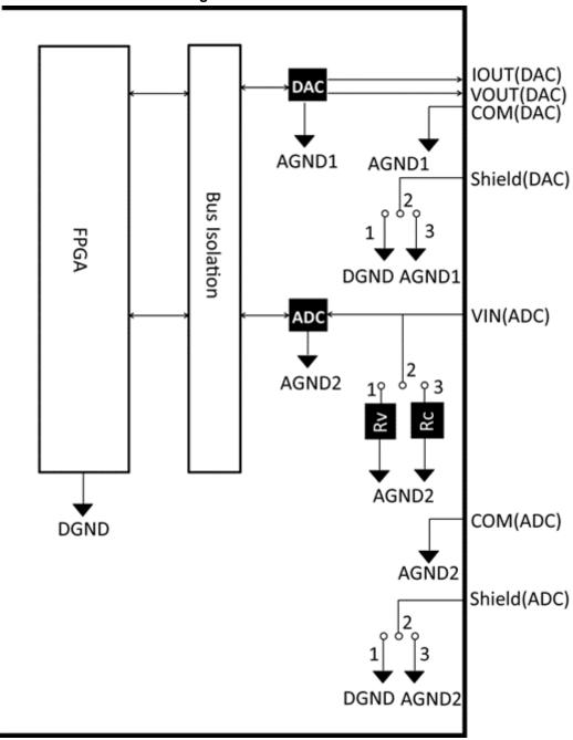
Rv: Voltage input terminating resistor (100 k $\Omega$ ), Rc: Current input terminating resistor
