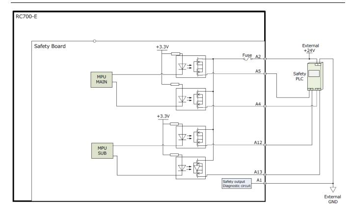
When Safety Relay is connected Insert a diode for circuit protection.
