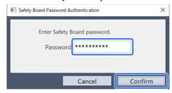
5. The contents of the settings to be written and the parameters sent to the Safety Board will be displayed. Make sure both settings are the same, and if there is no problem, click the [Confirm] button. By clicking the [Apply] button, the robot's set values and Hofs will be set on the safety board.
