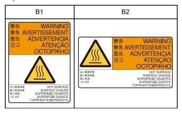
The surface of the Manipulator is hot during and after operation, and there is a risk of burns.
