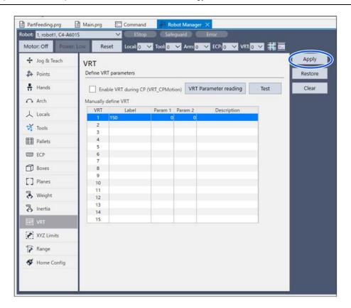
If the target motion (motion that you want to reduce vibration) is CP motion, place a checkmark on the [Enable VRT during CP] box.
