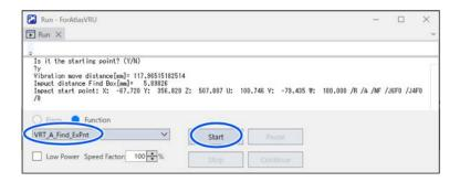
After confirming that the robot moves to the start position (P1 on the first figure of this section), click the [Start] button.
