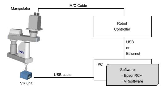
After reading the parameters and checking the effect of VRT, remove the VR unit and USB cable immediately. Do not operate the robot continuously with connecting the VR unit. (It is not a flex resistance USB cable. Parameters cannot be read unlimitedly.)
