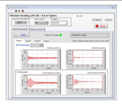
From the above operation steps, you can check the improvement effects of vibration when enabling VRT.
