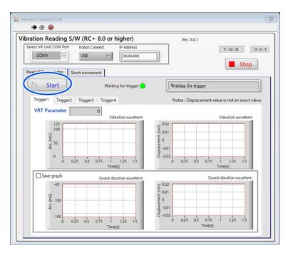
5. Confirm that the [Waiting for trigger] is lighted up in green and execute the program by Epson RC+. The program to be executed is the program that added "VRT Trigger" command according to the following steps.
