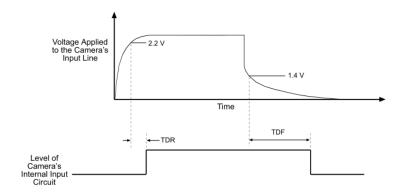
Time Delay Rise (TDR) = 1.3  $\mu$ s to 1.6  $\mu$ s Time Delay Fall (TDF) = 40  $\mu$ s to 60  $\mu$ s
