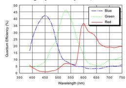
acA2500-20gc Spectral Response(From Sensor Data Sheet)
