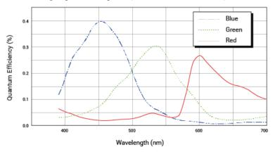
acA5472-5gc Spectral Response(From Sensor Data Sheet)
