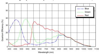
acA2500-14gc Spectral Response(From Sensor Data Sheet)
