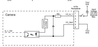
The inside is insulated by a photocoupler. Refer to the table below for the range of input voltage.
