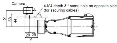
Dimensions of X and Y change depending on the position of the camera mid plate and the camera size. Refer to the table below for the values.
