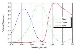
acA1600-60gc Spectral Response(From Sensor Data Sheet)
