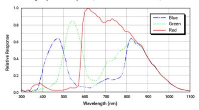
acA3800-10gc Spectral Response(From Sensor Data Sheet)
