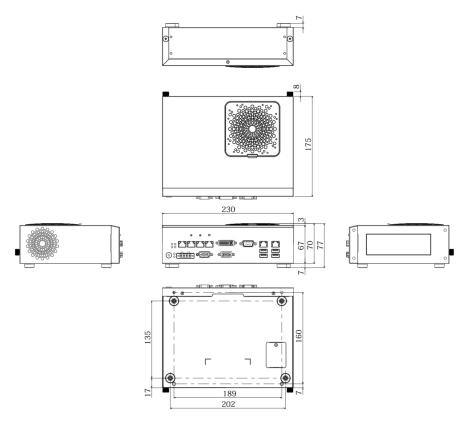
■ Install rubber foots for CV2-LB/SB/HB to respective positions.
