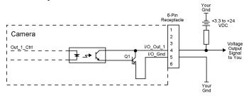
The following table shows the range of controlable voltage to the strobe output line. The maximum sink current is 50 mA.
