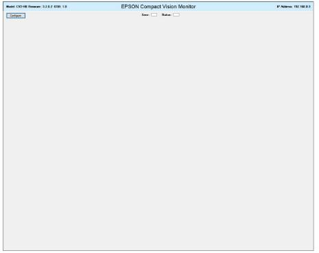
The states of the STATUS and ERROR LEDs located on the front panel are shown under the title bar.
