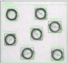
When using automatic multiple object search, if a child object can find multiple results, only one result can be found for each instance of the child object.
