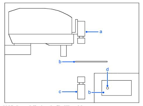
Mobile Camera Calibration using Fixed Upward Camera
