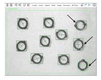
Image of 10 Rings with poor threshold settings
