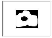
Figure D: Enlarged search window encloses two objects with the same gray scale value
