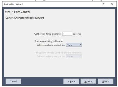
If you use lighting controls, specify a wait time before the lighting turns ON in milliseconds. Also, specify an output bit for turning ON the lighting.
