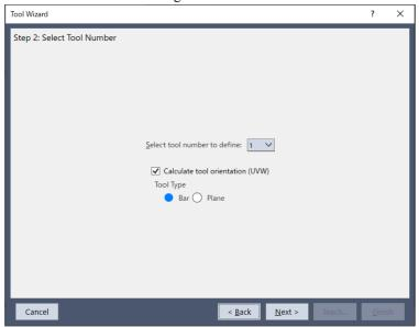
If you want to find the posture of the tool, check [Calculate tool orientation (UVW)]. Select either Bar type or Plane type as the tool type.
