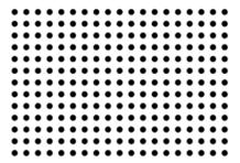
It is important to set the square lattice pattern so that it fills the entire field of view of the camera. If calibration is performed while the lattice pattern is in only a part of the field of view, distortion cannot be corrected properly since the area with no lattice pattern is not taken into account.
