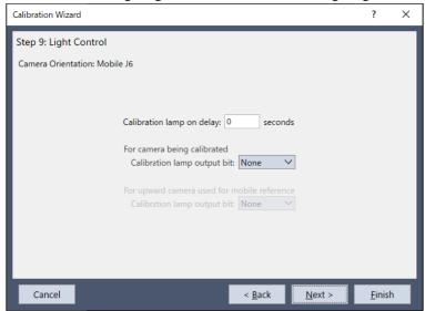
If you use lighting for the camera, specify a wait time before the lighting turns ON in milliseconds. Also, specify an output bit for turning ON the lighting.
