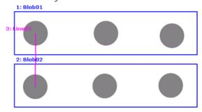
5. Run the sequence. A instance of the Line object will be created for each pair of results for StartPointObject and EndPointObject.
