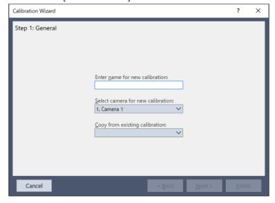
Enter the name for calibration in [Enter name for new calibration].
