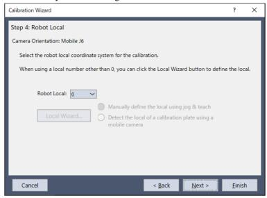
In this dialog box, you can run the local wizard to define local coordinate system to the local number. To run the wizard, select a local number other than "0", then click [Local Wizard...] button. Details of local setting using a camera are described in 7.7 Local setting using a camera.
