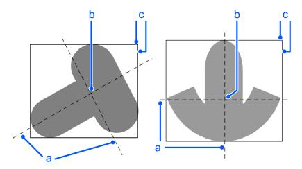
Principle axes, center of mass, and Extrema
