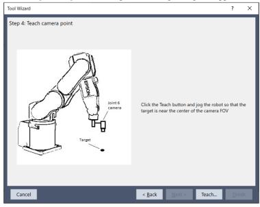
Jog the robot so that the target object can be detected near the center of the field of view.
