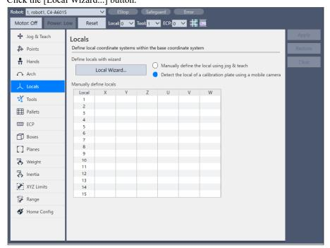
2. The [Local Wizard...] button appears when a robot local number other than "0" is selected in the step for selecting a robot local number in the calibration wizard. Click the button.
