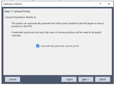
When [Automatically generate camera points] is selected: Multiple camera points are generated automatically by operating the robot automatically while detecting a target object in the FOV of the camera. The position of the target object in the FOV is detected for each camera point. When using the auto generation, it is necessary to teach a point where the target object is placed near the center of the FOV.
