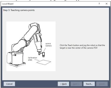
Jog the robot and move the center of the calibration plate to the center of the field of view.
