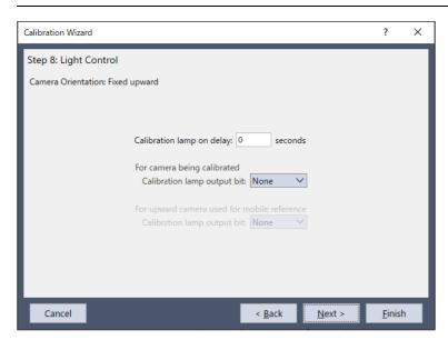
If you use lighting controls, specify a wait time before the lighting turns ON in seconds. Also, specify an output bit for turning ON the lighting.
