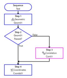
3. In you program, use VGet to retrieve coordinates from the Coordinates object. In this example, if Geom01 is Passed, then Geom01 coordinate results are copied to Coords01. If Geom01 is not Passed, then Corr01 executes. If Corr01 is Passed, then the Corr01 coordinate results are copied to Coords01. In the SPEL program, we can get the robot coordinates from Coords01:
