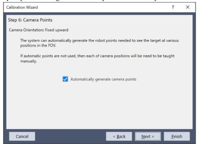
When the checkbox is selected: Multiple camera points are generated automatically by operating the robot automatically while detecting a target object in the FOV of the camera.
