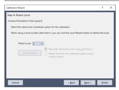
In this dialog box, you can run the local wizard to define local coordinate system to the local number. To run the wizard, select a local number other than "0", then click [Local Wizard...] button. Details of local setting using a camera are described in the following.
