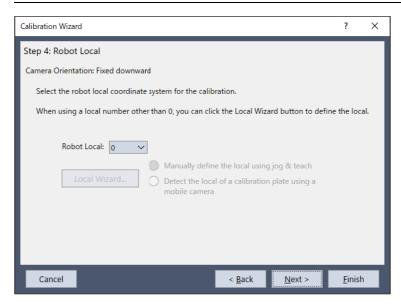
In this dialog box, you can run the local wizard to define local coordinate system to the local number. To run the wizard, select a local number other than "0", and then click the [Local Wizard...] button. Details of local setting using a camera are described in 7.7 Local setting using a camera.
