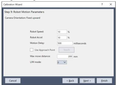
Set a speed and acceleration, and settling time after the robot motion (Motion Delay). To perform a fine calibration, set a slow speed and acceleration to ensure enough settling time.
