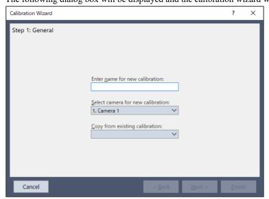
Enter the name for the new calibration. You can copy an existing calibration to specify the [Copy from existing calibration] after selecting the camera you will be calibrating.
