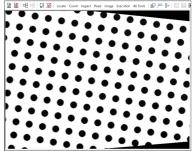
Example of image after correcting lens distortion and camera tilt
