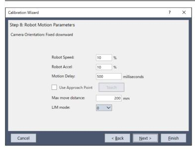
Set a speed and acceleration, and settling time after the robot motion (Motion Delay). To perform a fine calibration, set a slow speed and acceleration to ensure enough settling time.
