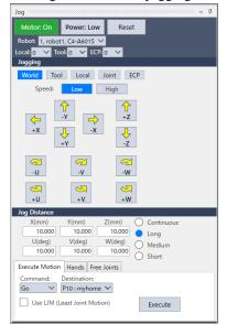
The Jog tab can be displayed by clicking the [Jog] button at the right side of the sequence and calibration trees. The Jog tab can be a fly-out panel.
