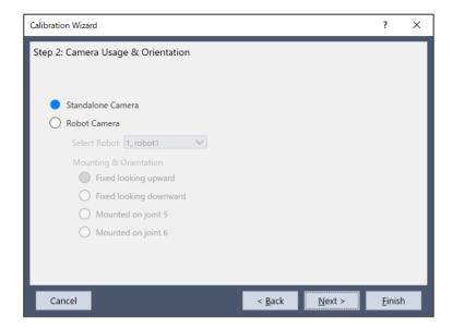
Step 2: Setting for calibration type and camera direction
