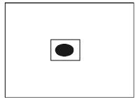
Figure C: Scene that cannot be segmented by gray-scale value
