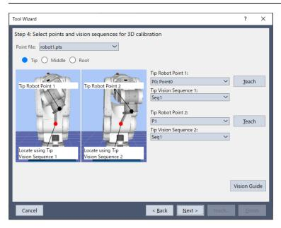
If [Calculate tool orientation (UVW)] is checked in Step2, select the tip, center, and root tabs and select the robot points and vision sequences in each tab.
