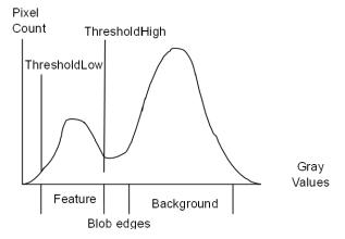
Setting the threshold values using a histogram
