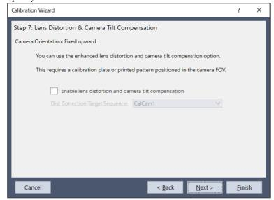
Selecting the checkbox enables correction. To correct distortion, it is necessary to create a target sequence for distortion correction in advance and specify it in this step.
