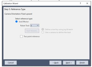
The reference point type for the fixed upward camera is [End Effector]. The reference point is a target on the tool mounted to the robot end effector. The target needs to be seen from the camera. (Although [Reference type] can be selected in this step, select [End Effector] for the fixed downward camera)
