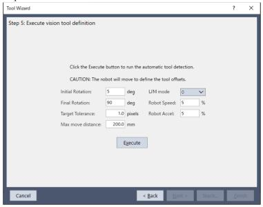
When using a fixed camera which is not calibrated, configure the following items. When calibrated fixed camera is used, setting is not necessary.
