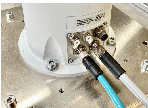
Connecting the manipulator and the controller.
