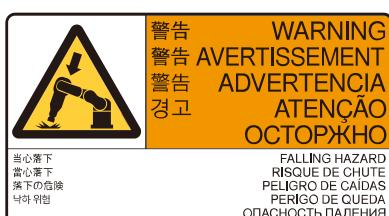
When releasing the brakes, be careful of the arm falling due to its own weight.
