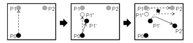
In the first Move, a trajectory from the initial position P0 to the target position P1 is planned (dashed line), and then the robot start motion. At this point, the robot moves to P1' because the path is corrected by the force control. (Solid line)
