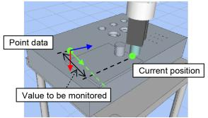
The orientation will be determined either by the angle between the axis (X, Y, or Z) specified by the Rot\_Axes property in the current tool coordinate system and the axis in the point data set for the DatumPoint, or by the amount of rotation of arbitrary axis. If X is the specified axis, this will determine the angle between the X axis of the specified point data, and the current X axis as shown in the diagram below.
