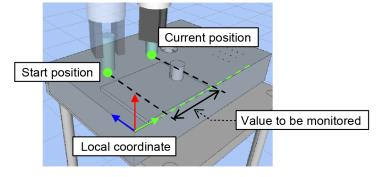
The orientation will be determined either by the angle between the axis (X, Y, or Z) specified by the Rot\_Axes property in the current tool coordinate system and the axis in the tool coordinate system at the start of
