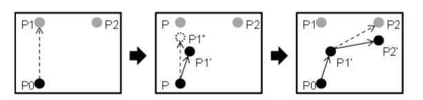
In the first Move, a trajectory from the initial position P0 to the target position P1 is planned (dashed line), and then the robot start motion.
