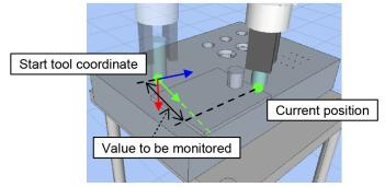
The orientation will be determined either by the angle between the axis (X, Y, or Z) specified by the Rot\_Axes property in the current tool coordinate system and the axis in the tool coordinate system at the start of monitoring, or by the amount of rotation of arbitrary axis. If X is the specified axis, this will determine the angle between the X axis at the start of monitoring, and the current X axis as shown in the diagram below.
