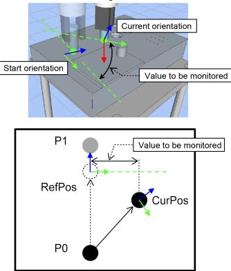
The orientation will be determined either by the angle between the axes (X, Y, or Z) specified by the Rot\_Axes property in RefPos and CurPos, or by the amount of rotation of arbitrary axis. If X is the specified axis, this will determine the angle between the X axis for RefPos and the X axis for CurPos as shown in the diagram below.
