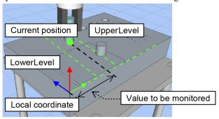
The orientation will be determined either by the angle between the base coordinate system or the local coordinate system used as the basis for robot positions and the axis (X, Y, or Z) specified by the Rot\_Axes property in the tool coordinate system, or by the amount of rotation of arbitrary axis. If X is the specified axis, this will determine the angle between the X axis in the reference coordinate system and the X axis in the current tool coordinate system as shown in the diagram below.
