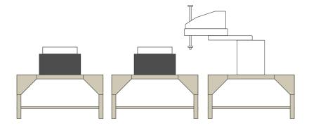
It is important that the camera is not affected by the vibrations of the flexible feeder or another moving device. If the vision system is affected by residual vibrations, unreliable coordinate data sent to the robot may compromise the precision of the whole system.
