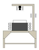
Good example: Vibrations from a flexible feeder do not interfere with the camera
