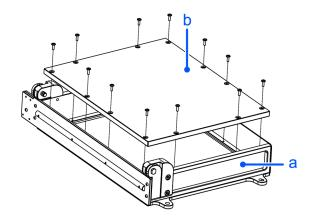
Mounting screw x 12 Tightening torque: 1.2 N⋅m
