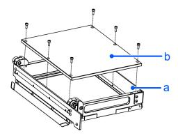
Mounting screw x 7 Tightening torque: 1.2 N⋅m
