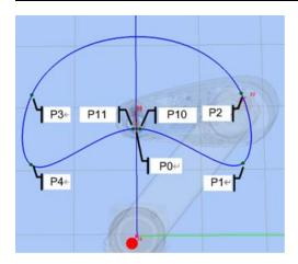
It is Open Curve but the start point and end point connect smoothly by going through P10 and P11.
