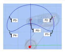
Because it is Closed Curve, the start point and end point connect smoothly.
