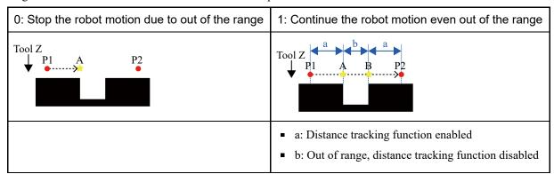
When the parameter is set to "1" and the robot moves outside of the range, the robot moves on the trajectory from the start point (P1) to the target point (P2) with CP motion. As shown in the figures below, the trajectory between A and B (outside of the available range) will become parallel to its of P1-P2. When the robot arrived to point B, the robot returned to inside the available range. Therefore, the robot is controlled based on the measured value and may move suddenly.
