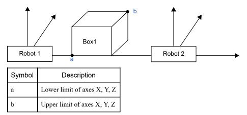
Configure the Box 1 from Robot 1 position
