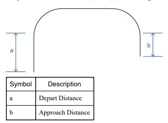
There are a total of 8 entries in the Arch Definition Table with 7 of them (0-6) being user definable. The 8th entry (Arch 7) is the default Arch which actually specifies no arch at all which is referred to as Gate Motion. (See Gate Motion diagram below) The Jump instruction used with the default Arch entry (Entry 8) causes the arm to do the following:
