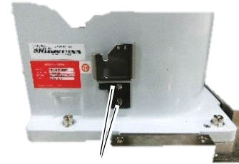
Hexagon socket head cap bolt 2-M4×10
