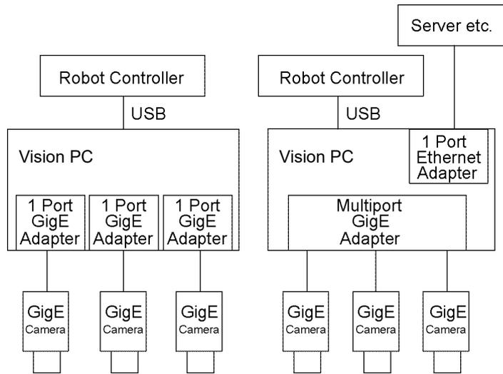
The main advantage of the peer-to-peer connection is that it can make full use of the network bandwidth for transferring captured images from each camera due to independent network. This allows you to get great performance of each camera and to design the system easily. The peer-to-peer connection is particularly effective when using multiple cameras in the external trigger mode.
