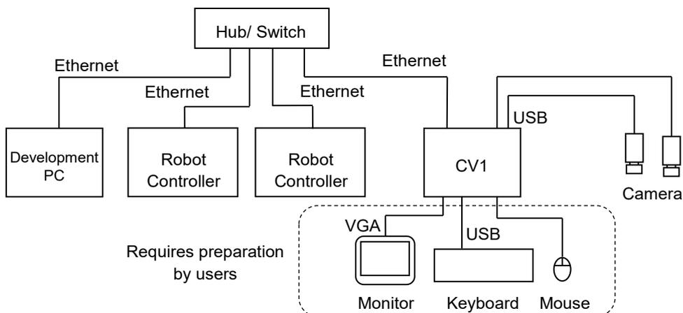
NOTE: The project numbers for the CV1 should be set to the projects transmitted to each Robot Controller without duplication.
