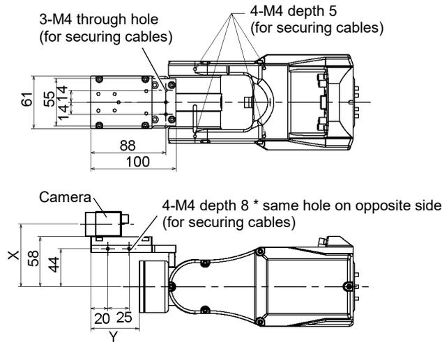
Dimensions of X and Y change depending on the position of the camera mid plate and the camera size. Refer to the table below for the values.
