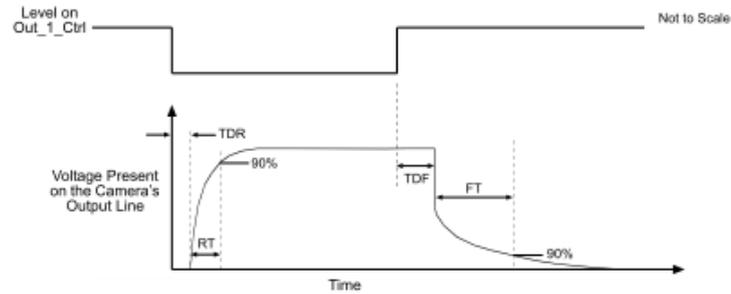
Fig. 40: Output Line Response Times
