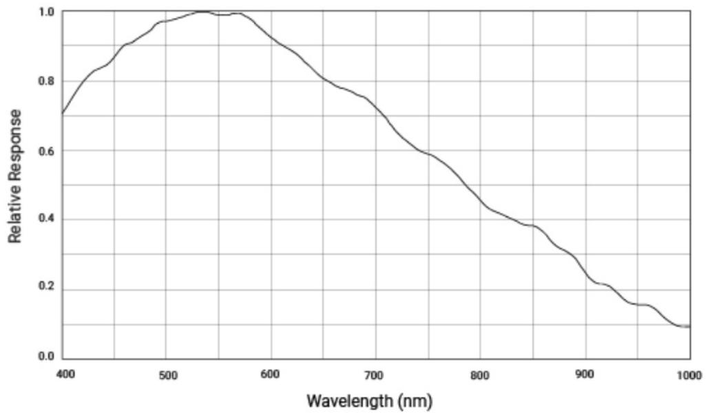
4.2.7 CCD/CMOS Spectral Characteristics of Color Camera
