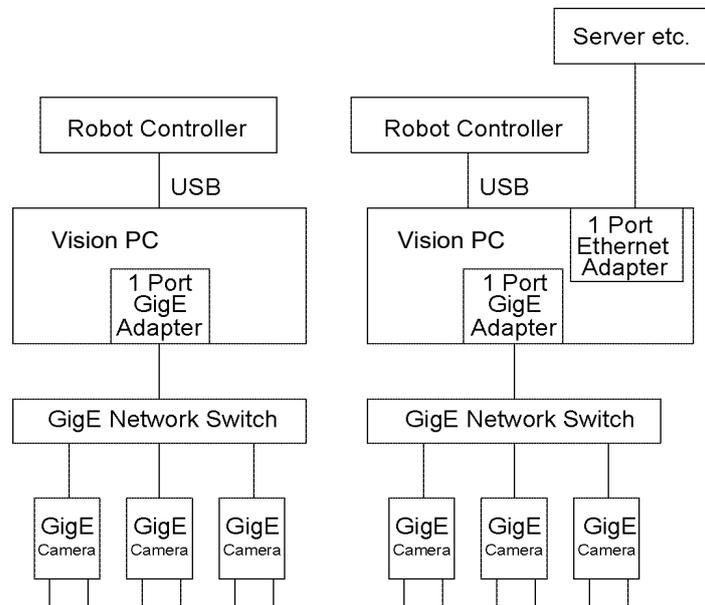
This network configuration is effective for systems where there are a lot of cameras or where GigE cameras are set away from the Vision PC. However, this configuration may not be able to improve the system performance because the imaging timings must not be overlapped.
