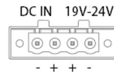
Appropriate Wire Diameter :AWG14 to AWG24
