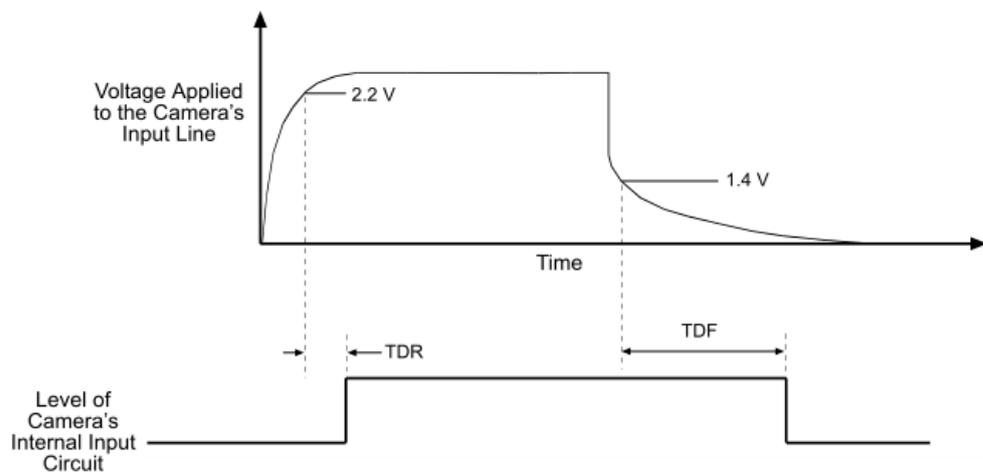
Time Delay Rise (TDR) = 1.3 μs to 1.6 μs
