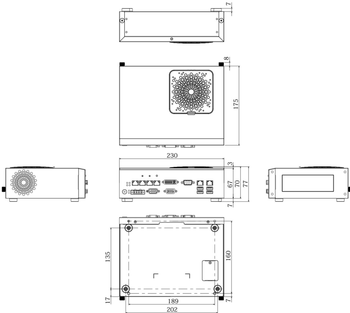
\* Install rubber feet for CV2-LB/SB/HB to respective positions.
