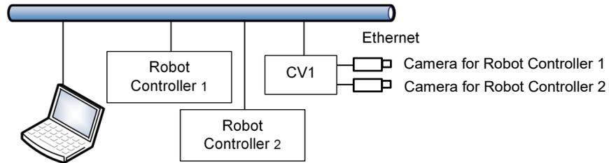
(1) Connect an Ethernet cable between the camera, the Controller, and the PC.
