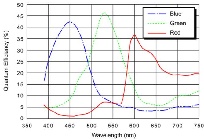
acA2500-20gc Spectral Response(From Sensor Data Sheet)
