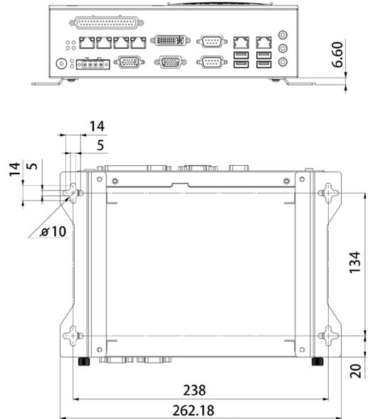
Brackets installed on the side
