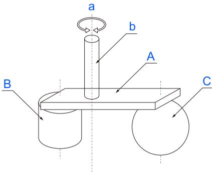
$$\text{Whole moment of inertia} = \text{Moment of inertia of end effector(A)} + \text{Moment of inertia of work piece(B)} + \text{Moment of inertia of work piece(C)}$$
